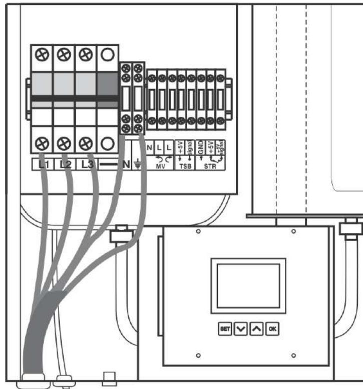
Pav. 7: Connecting diagram of the electric cables
